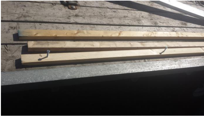
#56: ensure the screws are in the 1x2 to prepare for fastening the cover to the base
