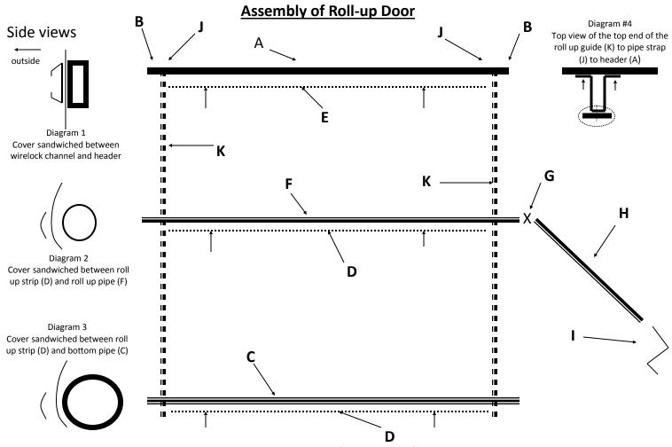
This is the order that assembly must be done. Refer to parts list for material lengths and names
